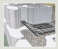
It's Versatile... Variable setbacks, sharp radius turns, "One Unit" construction, and complete interchangeability are all features of Rockwood's Legend System. The ability to mix various sizes and colors within a wall enhances your imagination without sacrificing structural integrity. Plus, the Anchor Bar allows you to build at any setback you desire – from 0° to 14°, providing the only "true" vertical setback in the industry.
